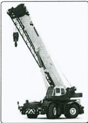
Over 40 Ton Telescoping Boom Crane
